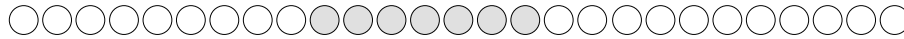
Figure 10.5: The sequence splitting method of parallel random number generation. There is one stream of random numbers and each process gets a consecutive sequence of this stream by taking the next n values from the stream. The value of n is determined by the application.
