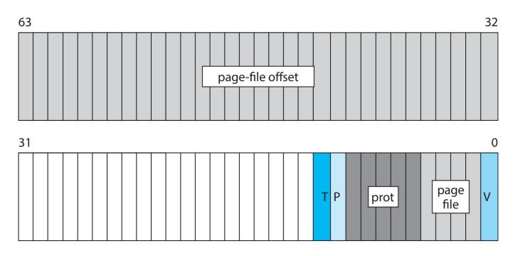
5 bits for page protection, 32 bits for page-file offset, frame address, 4 bits to select a paging file, and 20 bits for additional bookkeeping
