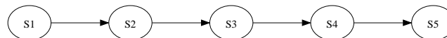
Figure 1.5: A data dependence graph exhibiting no parallelism. The tasks must be performed one after the other, from left to right.
